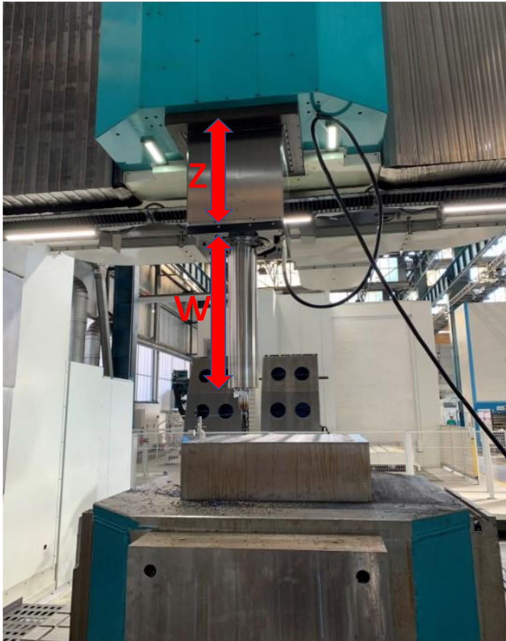
Figure 16. The axes where stiffness variation realized
