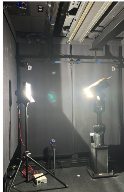
(b) Tango mock-up illuminated by a sun lamp.
