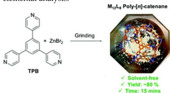
Figure 2.1: Mechanochemical synthesis of [(ZnBr 2 ) 12 (TPB) 8 ] poly-[ n ]-catenanes [4]
