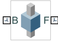
Figure 52 Prismatic joint block
