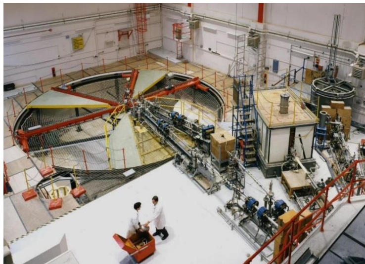
Figure 3.9 – Irradiation hall at NPL facility, where it is possible to see the end of the beamline and the target zone. (Source: Castiñeira, S.-, Göök, A. B., Vidali, M., Hawkes, N. P., Roberts, N. J., Taylor, G. C., & Thomas. (2020.). Towards the adoption of ^{238}\text{U}(n,f) and ^{237}\text{Np}(n,f) as primary standards for fast neutron energies Welcome to the National Physical Laboratory.)
