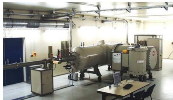
Figure 3.3 – Tandem accelerator: A) sketch of the general structure; B) a real picture. (Source Bolzonella, M. (2019). Characterization of a passive dosimeter based on a CR-39 track detector for environmental and personal dosimetry in neutron mixed fields. Politecnico di Milano.)
