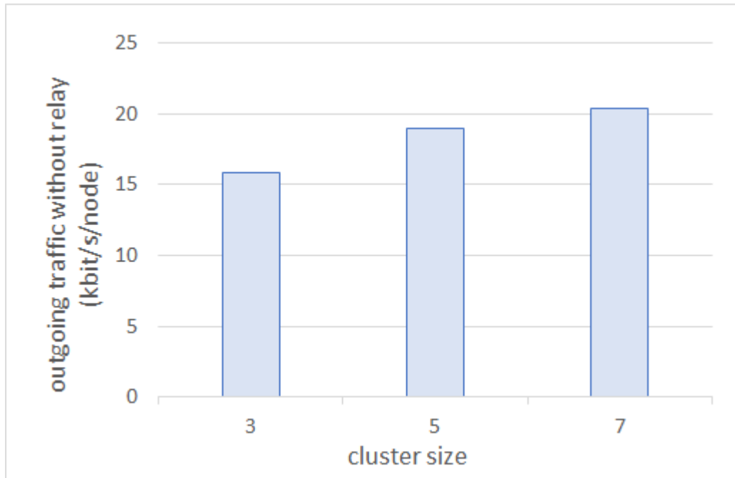
Figure 5.4: Heartbeat mechanism overhead using Raft default timings: one heartbeat every 50 ms.
