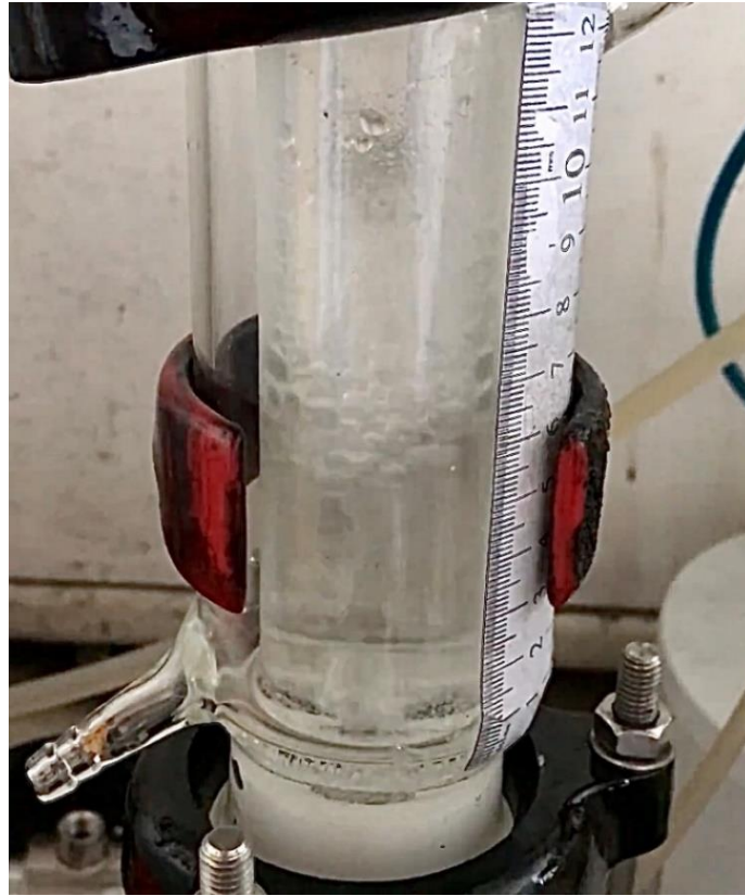
Figure 29: Screenshot of the variation of foam formed on the free surface of the mixture 3
