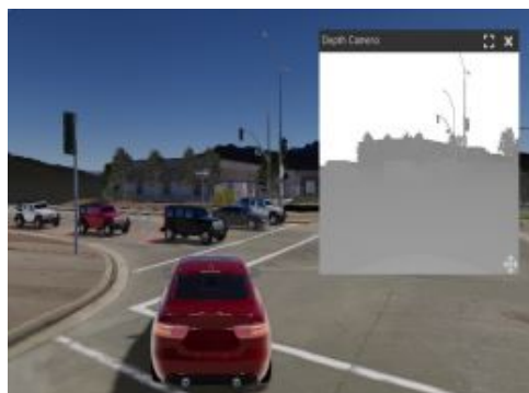
Figure 2.6: Depth camera sensor output example.
