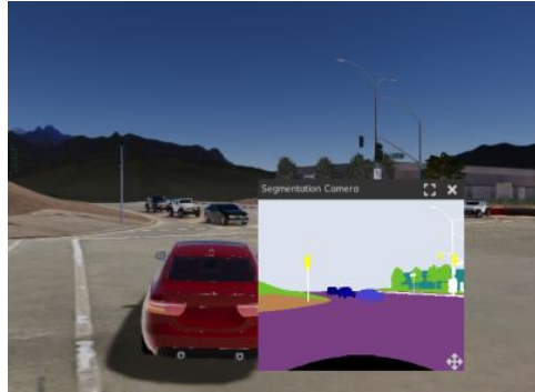
Figure 2.7: Semantic segmentation camera sensor output example.
