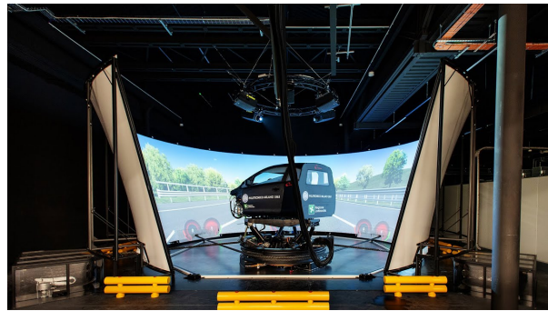
(b) DiM400 driving simulator installed in Politecnico di Milano, Bovisa campus.
