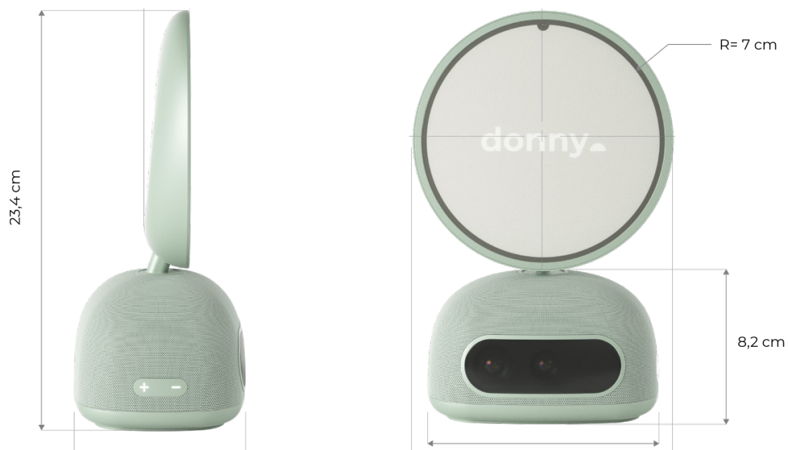
Figure 14. Donny dimensions. The device has been designed as compact as possible without sacrificing the usability of the interface.
