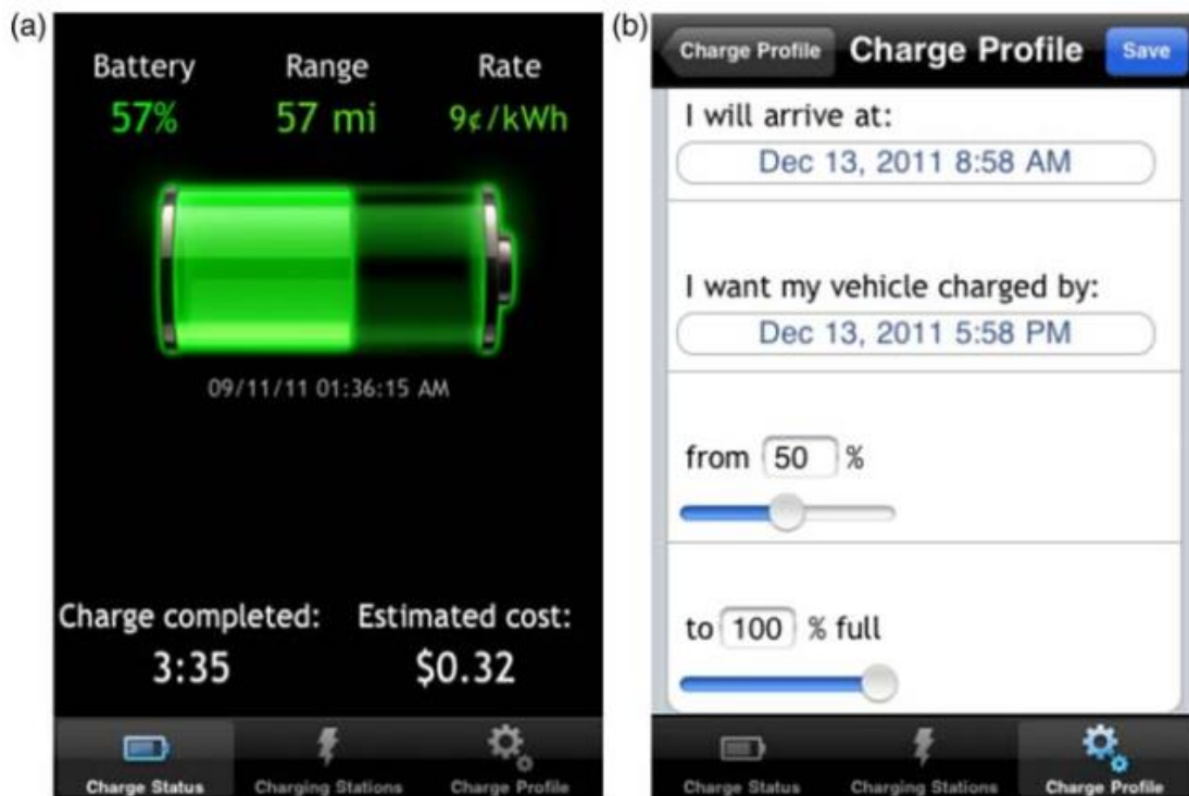
Figure 39: (a) Charge status screen. (b) Charge profile screen (Mal et al., 2013).
