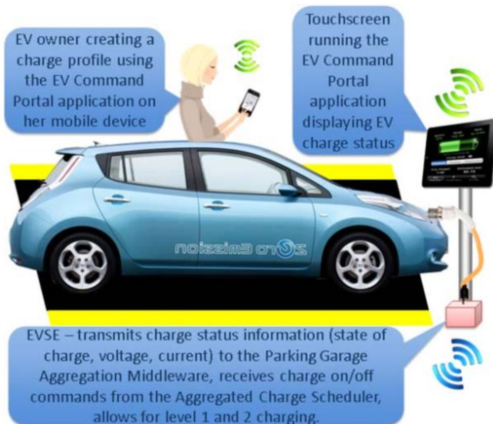
Figure 38: Charging station equipment and activities (Mal et al., 2013).
