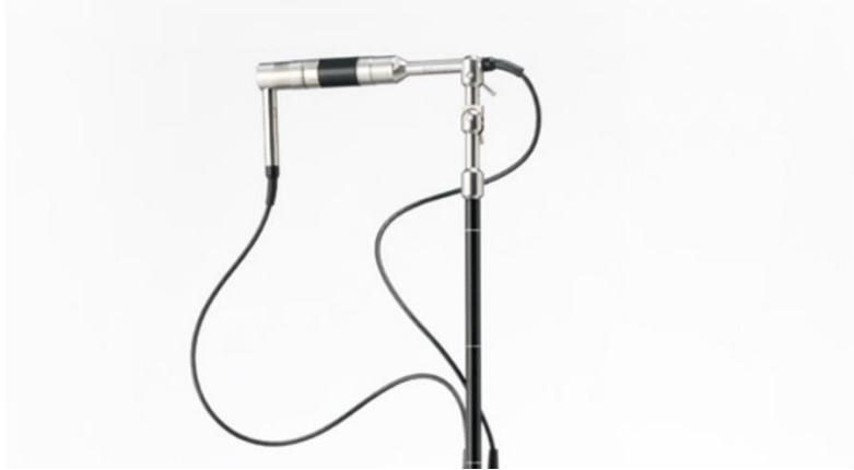
Figure 26 - Sound intensity probe
