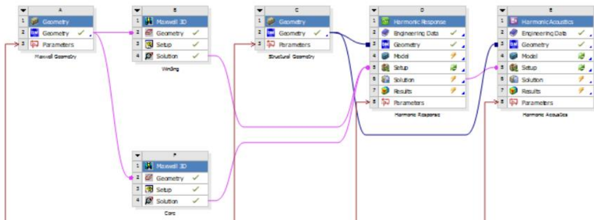
Figure 72 - Complete Workflow for acoustic analyses
