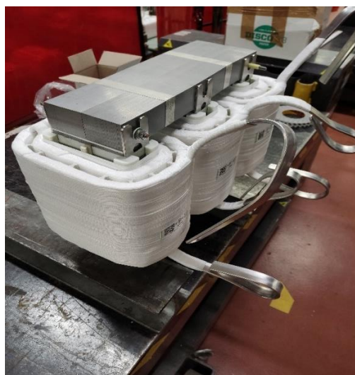
Figure 3 - Winding with the presence of cooling channels (in white)
