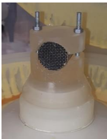
Figure 2.10: New spin-coating sample holder
