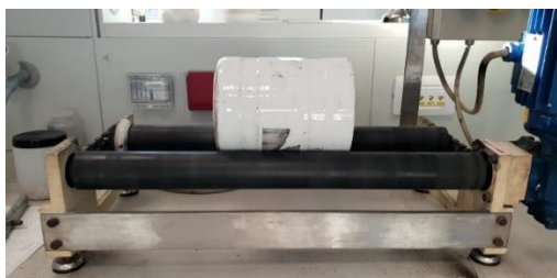
Figure 2.5: Ball milling process
