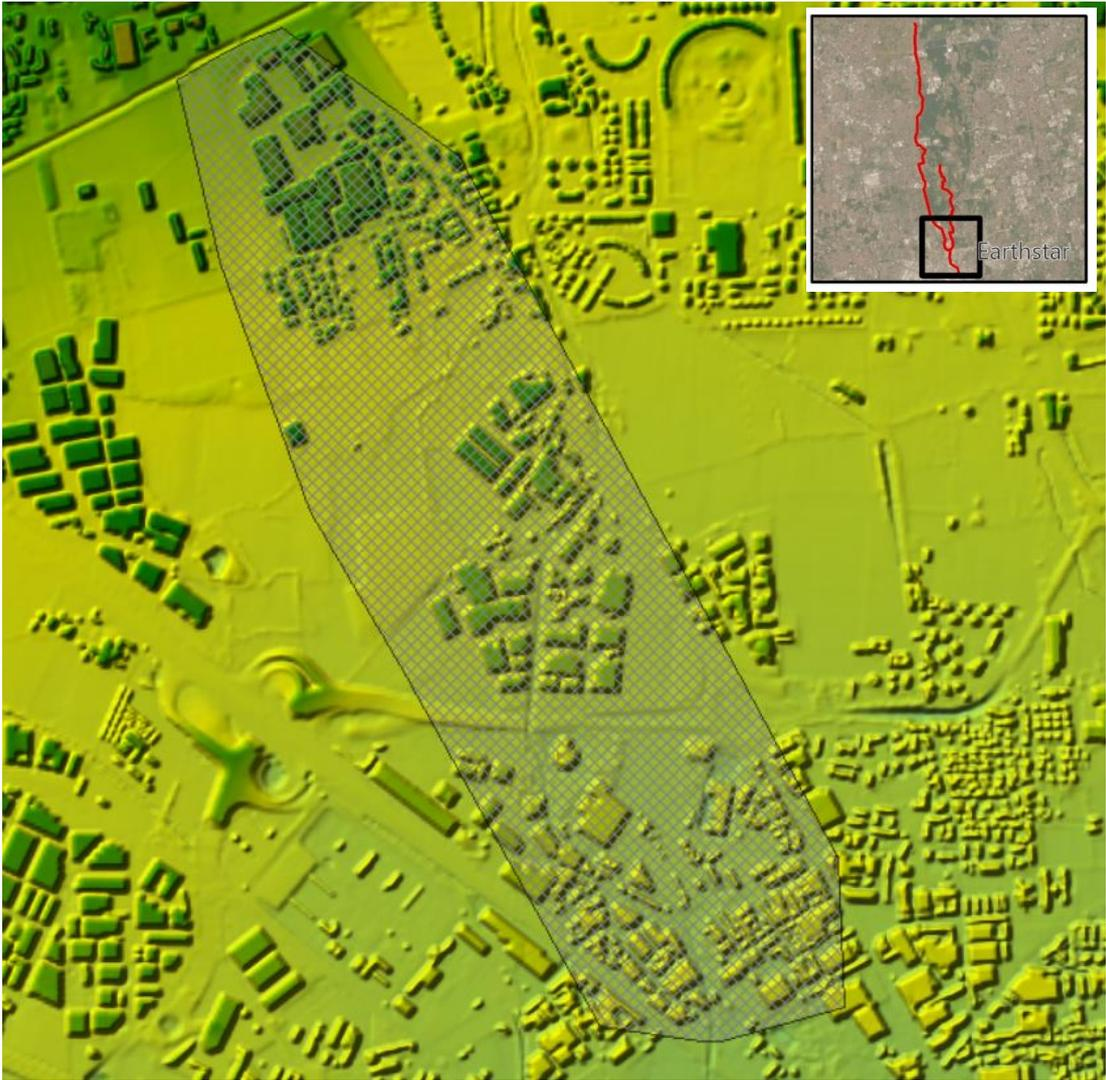
Figure 3.20: Example of terrain and computational mesh representation (Guisa downstream)
