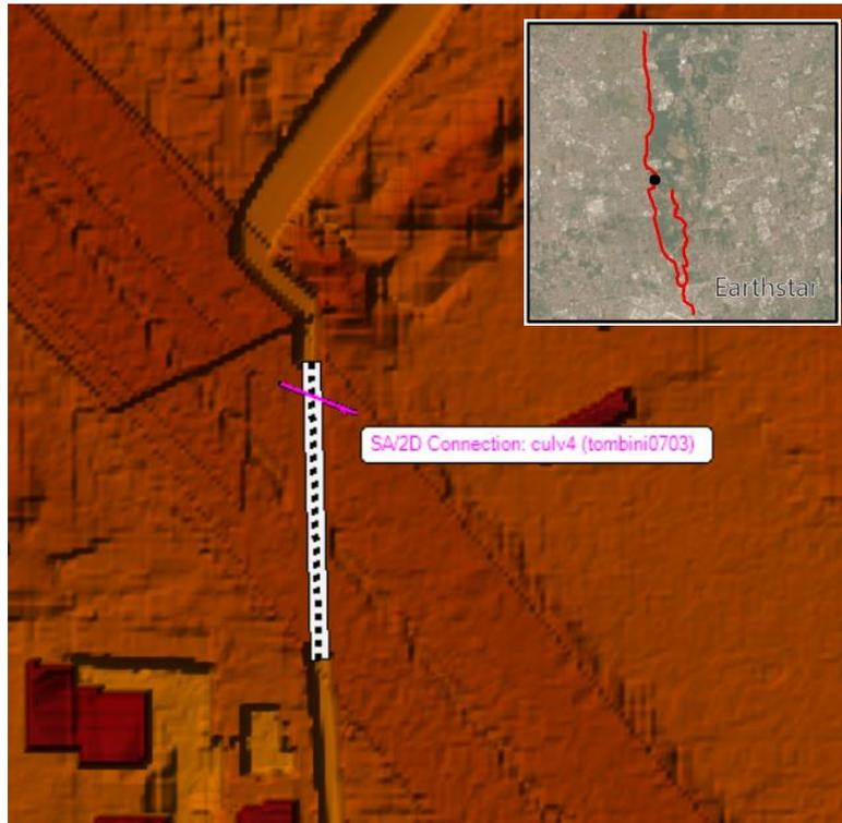
Figure 3.27: Culvert 4 - RAS Mapper
