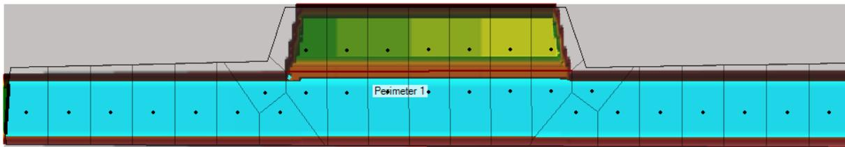
Figure 4.57: Cell size 3 meters with break line
