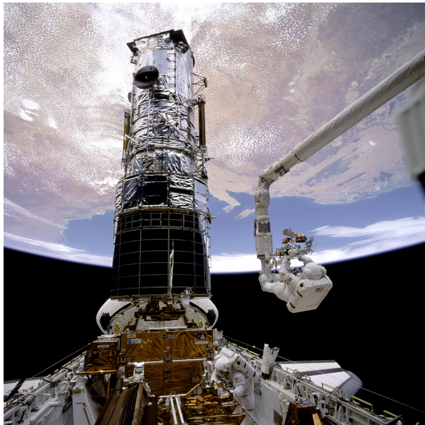
Figure 1.2: The first servicing mission to the Hubble Space Telescope saw astronauts install a set of specialized lenses to correct the flawed main mirror in the telescope. Credits: NASA
