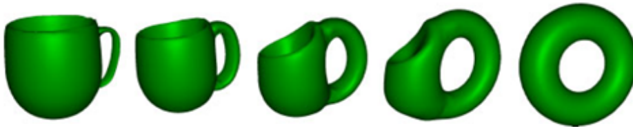
Figure 3.4: Taken from [45], a representation of morphing procedure applied to triangular meshes: from a mug shape, a torus shape is obtained.
