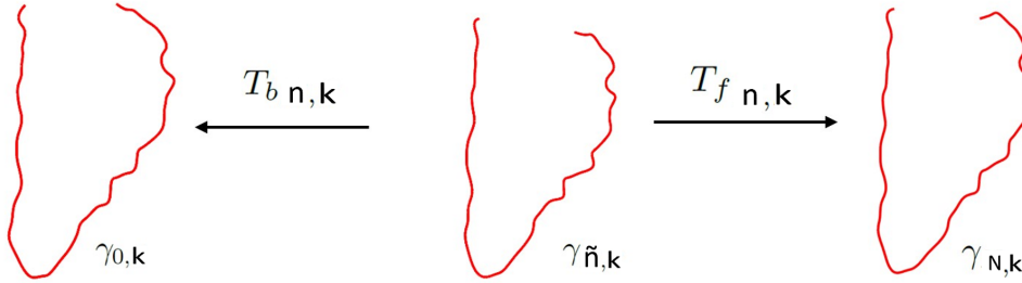
Figure 3.2: Scheme of application of the forward and backward transformations, respectively T_{f_{n,k}} and T_{b_{n,k}} , in the procedure for automatic registration (see Section 3.2) of contours \gamma_{n,k} (red lines). The backward transformation is applied for each k with n varying from \tilde{n} back to zero. The forward transformation instead for each k is applied with n varying from \tilde{n} to the maximum value, N .
