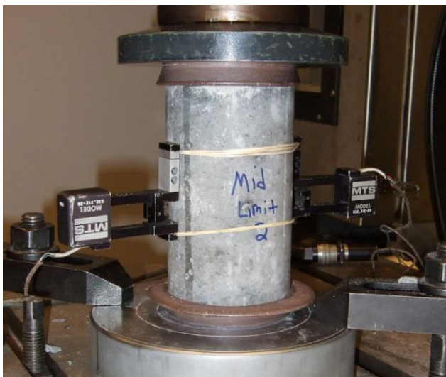
Figure 4.8 Uniaxial compression test on a cylindrical concrete sample and its schematic replication. Sources:
