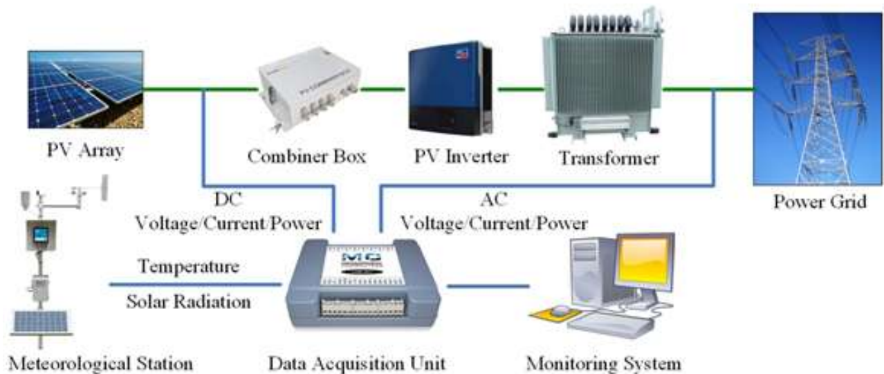
Figure 12. A system for monitoring the on-grid PV system with an online interface [21].
