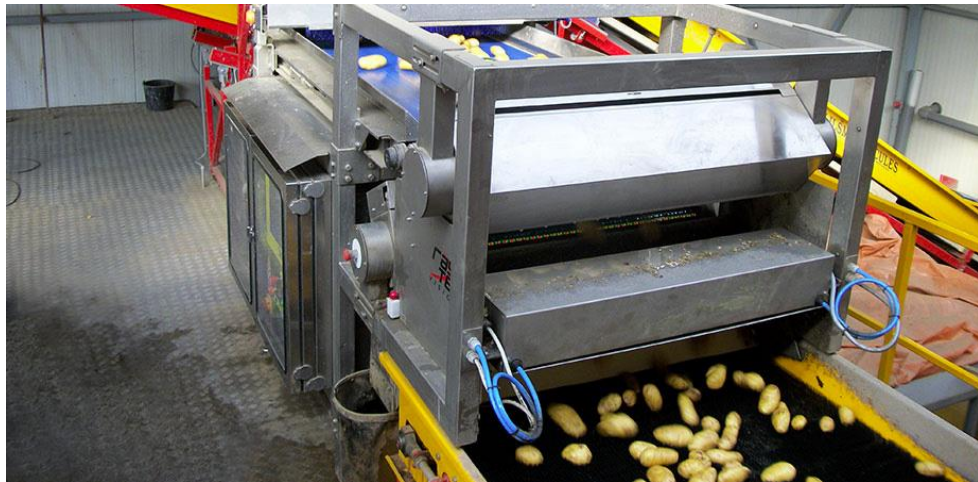
Figure 2 - An installation dedicated to the control of peeled and unpeeled potatoes thanks to NIR technology
