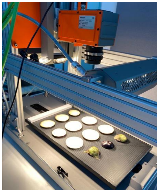
Figure 9 - Dark current calibration and image acquisition setting
