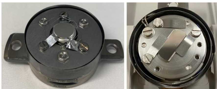
Figure 2.28: MBE system sample-holders for different monocrystal’s shapes. The visible filaments are the thermocouples. On the left, there is an EB-heater, while on the right a resistive heater.
