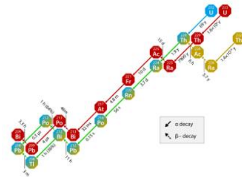
Figure 19: The figure shows the decay chains of U-232 and U-233 (m for months) [36].
