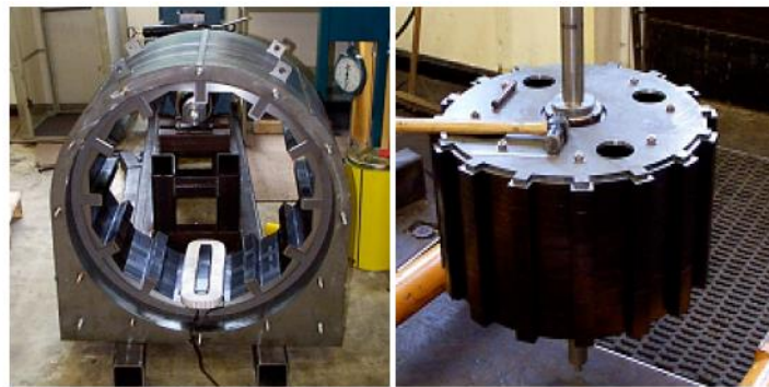
Figure 15 Stator and rotor of the 20kW switched reluctance machine
