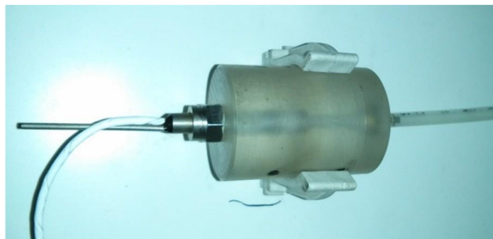
Figure 13 - Picture of a Kulite type pressure transducer
