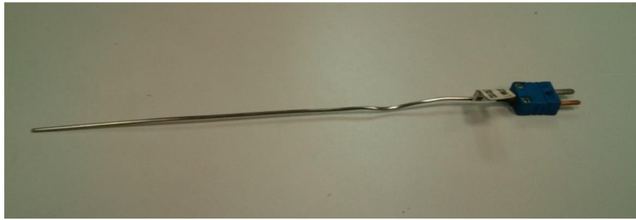
Figure 12 - Type T (copper-constantan) thermocouple
