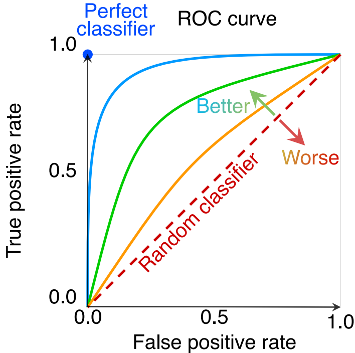
Figure 4.3: Depiction of some examples of ROC curves. A higher value of AUC indicates a better classifier. The random classifier corresponds to the red dashed line
