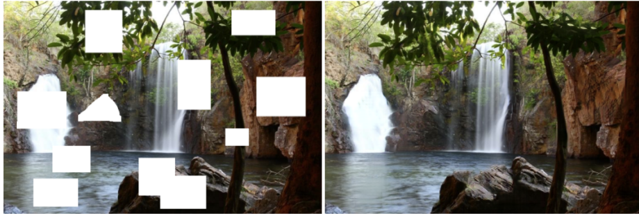
Figure 3.2: An example of inpainting taken from [66]: on the left an input image with missing pixels, on the right the inpainted version of the image where those pixels were reconstructed.
