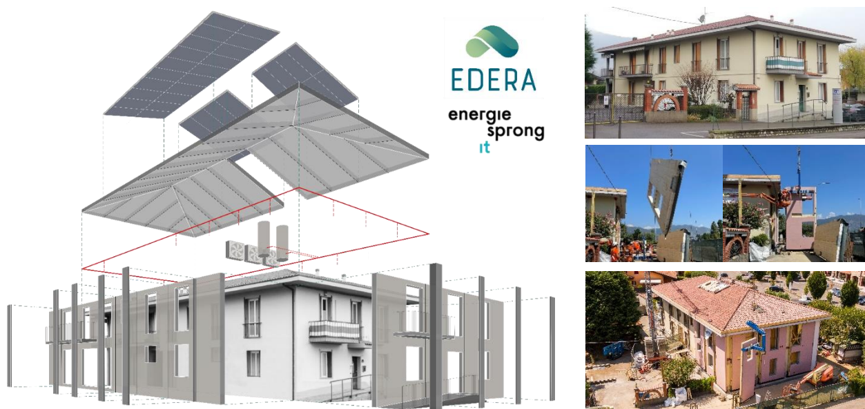
Figure 15 First Energiesprong project in Italy: 3D scheme with pictures before and during the renovation
