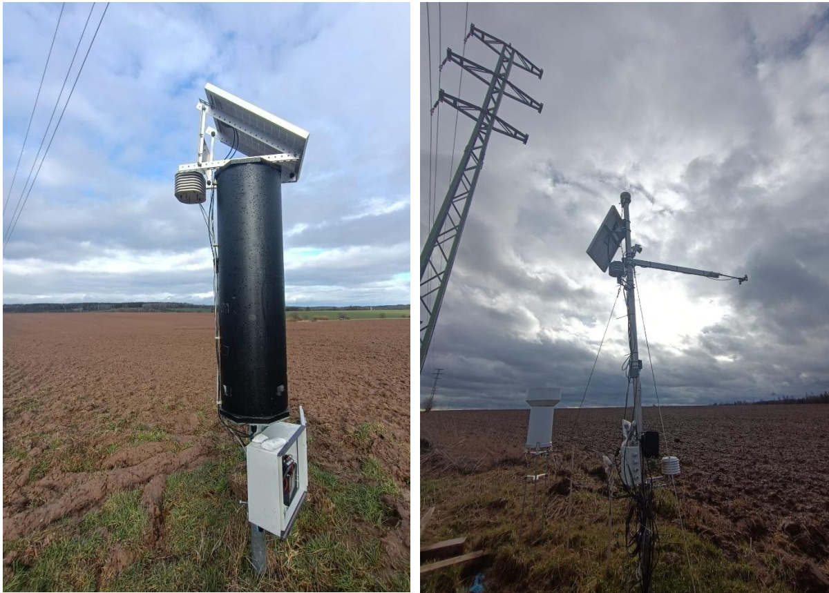
Figure 6 – (a) CRNS station, (b) Meteorological station near CRNS.
