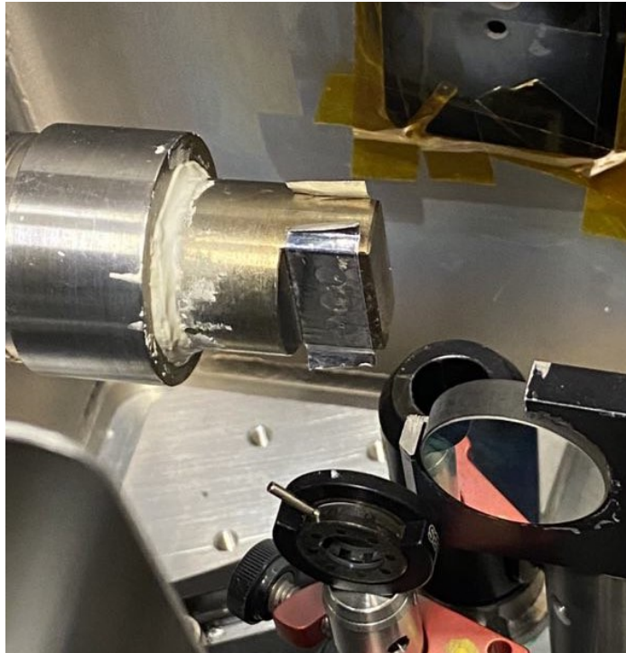
Figure 2.2: Cell used in our experiments for the HHG through Argon.
