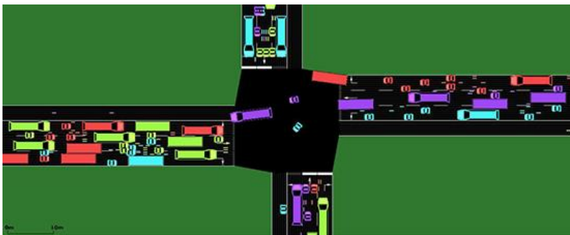
Fig. 22. Birds eye view of the cars and buses in the graphical user interface of SUMO
