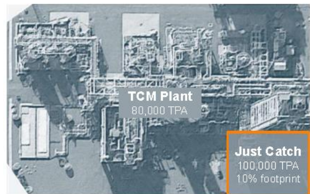
Figure 2.3 Aker solution's Just Catch new modular pilot plant compared to TCM.
