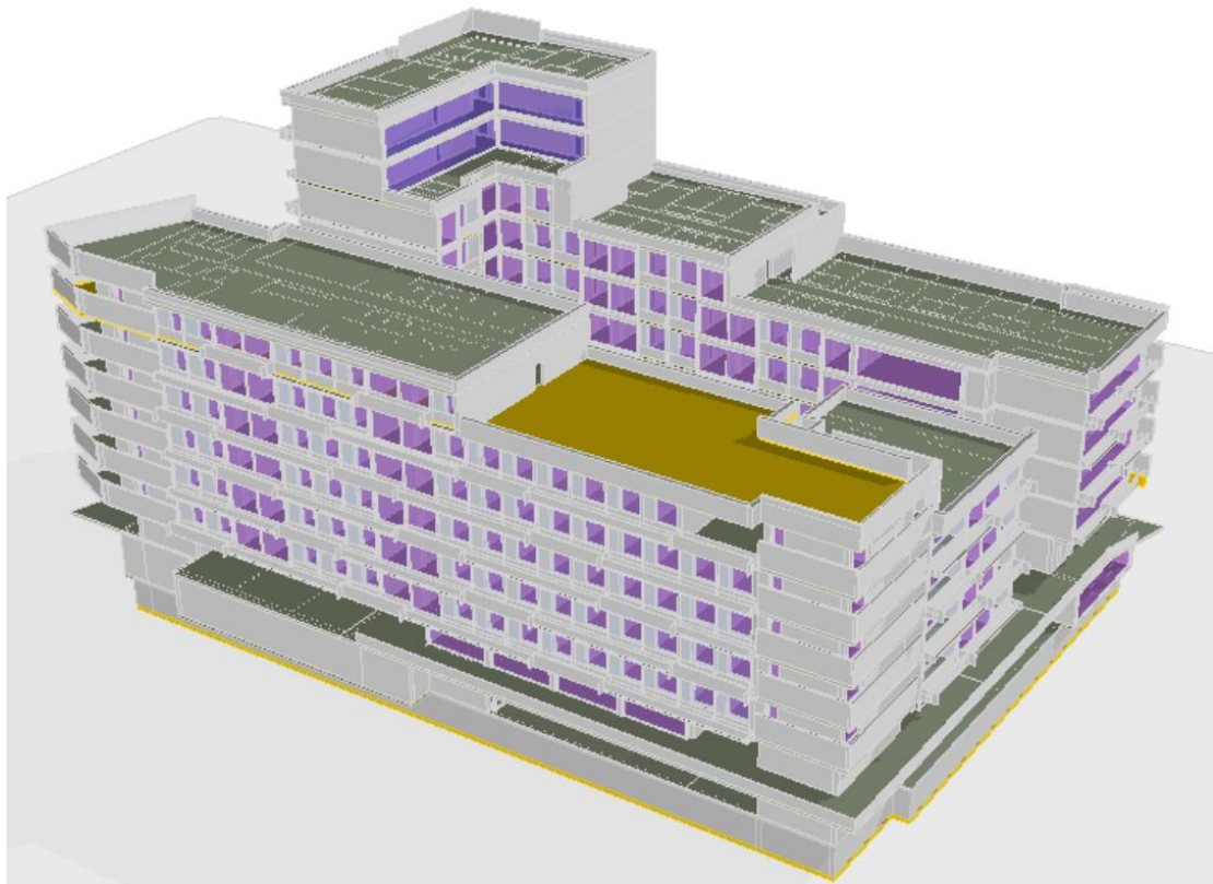
Figure 73. The 3D result of the energy model in Termolog
