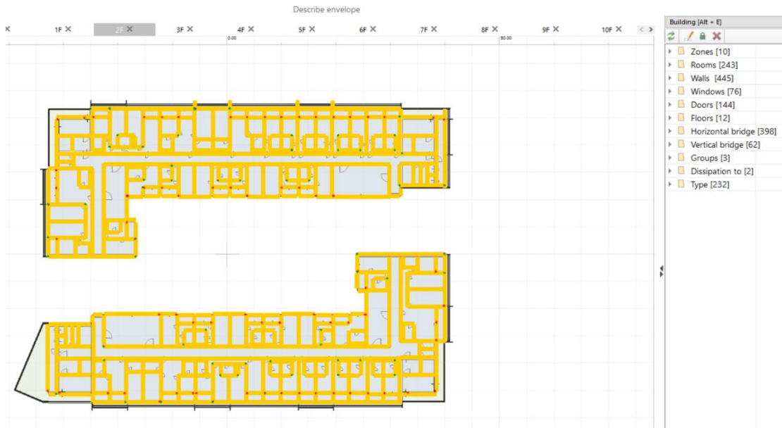
Figure 72. The 2D plan with different components in Termolog
