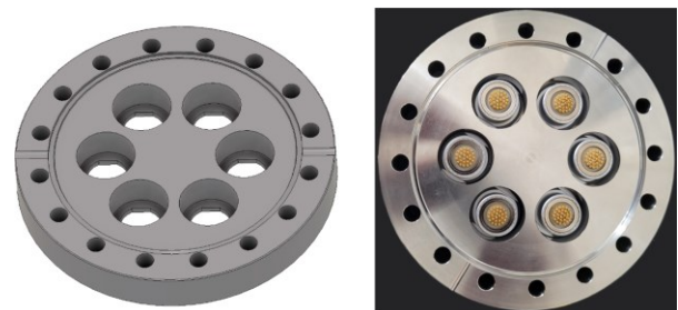
Figure 4.2: 3D model of the flange (left). Picture of the six 27-pin connectors mounted on the flange (right).
