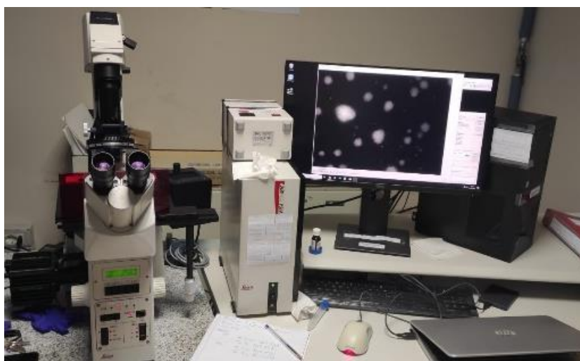
Figure 3.12: Confocal microscope (Leica DM IRE2) used for thrombus height and volume evaluations.
