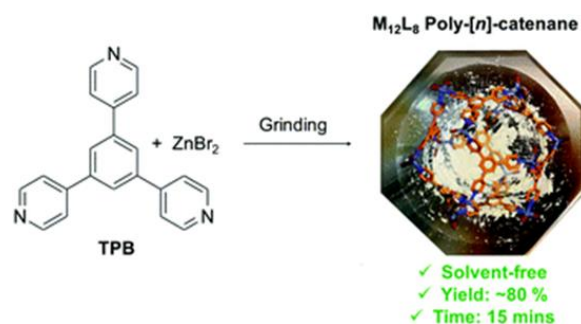
Figure 2.1: Mechanochemical synthesis of a1 phase [73]
