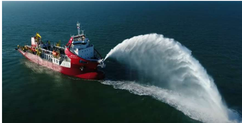
Figure 4.1: TSHD during rainbowing process.
