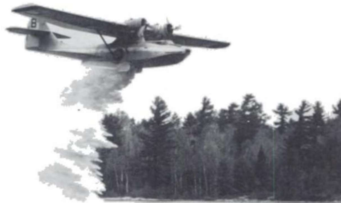
Figure 5.1: Example of limestone application by firefighting aircraft during a lake liming operation (Olem, 1991).
