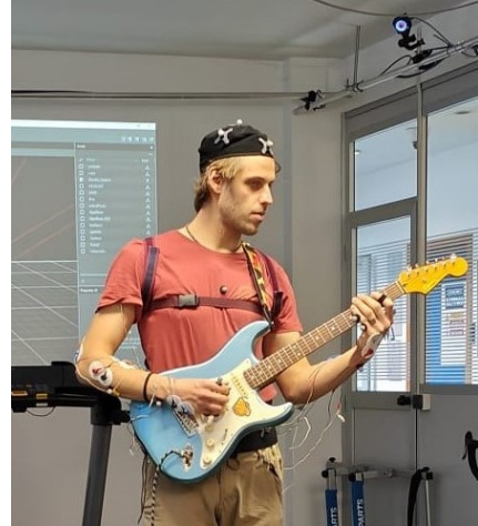
Figure 2: Guitarist during the acquisition session with electrode pads placed on arms.
