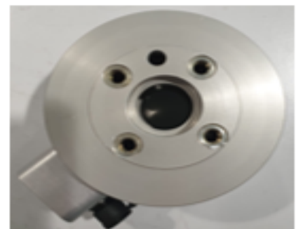
(b) 6-axis strain gauge cell. It was tested for frequency response
