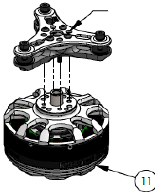
Figure 1.25: Mounting the adapter on motor (Picture from [4])
