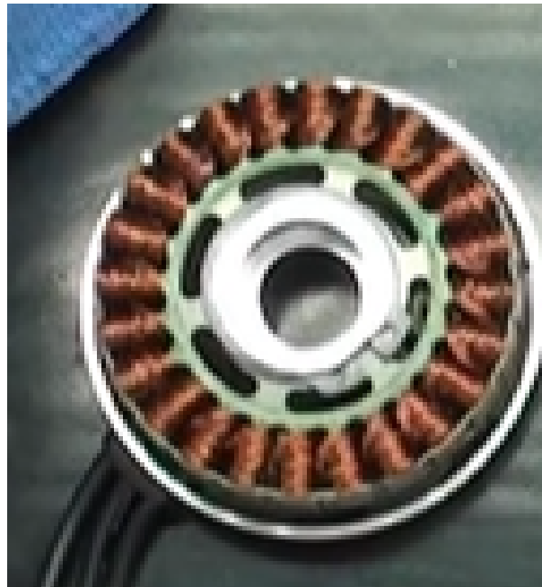
Figure 1.9: Stator, front view (pictures from 1.9 to 1.14 are from KDE Direct)
