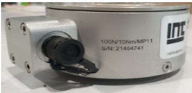
(b) 6-axis strain gauge cell. It was tested for frequency response
