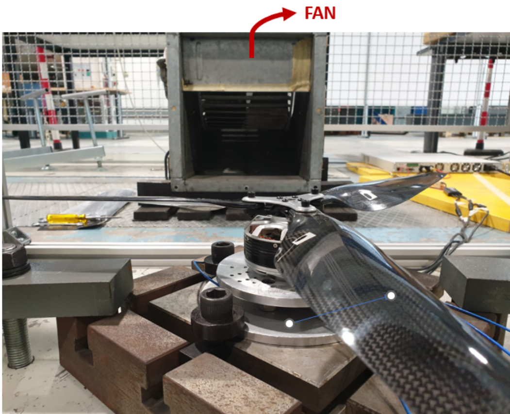
Figure 4.2: Piezoelectric system for measuring LTU loads
