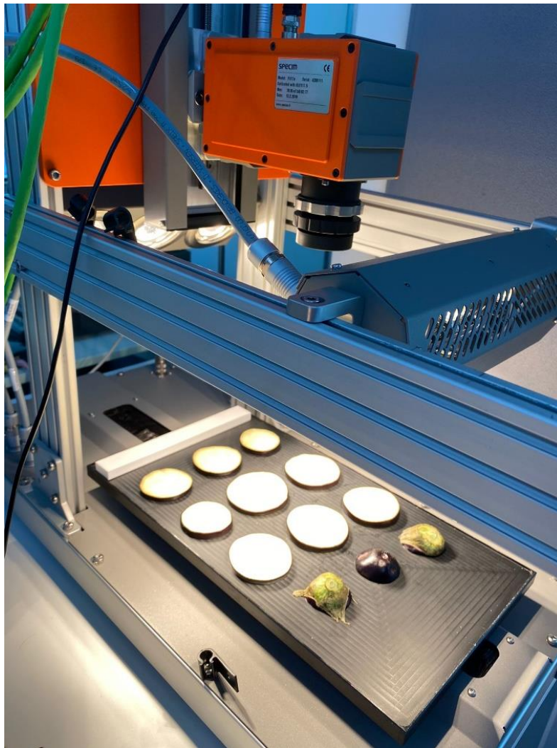
Figure 7 - Dark current calibration and image acquisition setting
