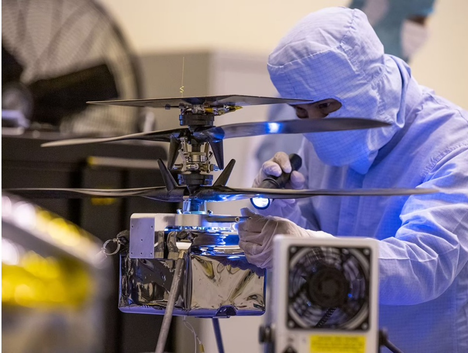
Figure 1.8: NASA technician is shown working on Ingenuity that features a Kapton insulation blanket protecting the Helicopter Warm Electronics Box
