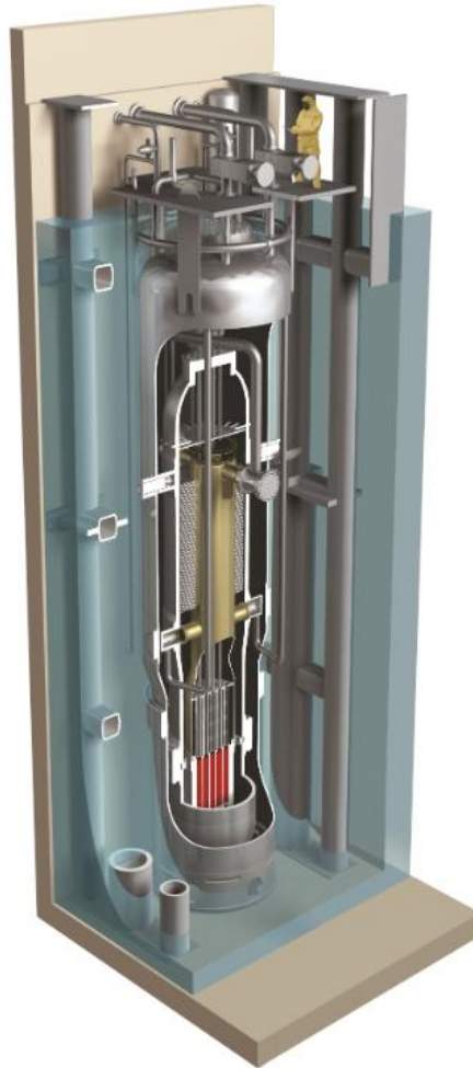
Figure 5: 3-D rendered view of a NSSS module
