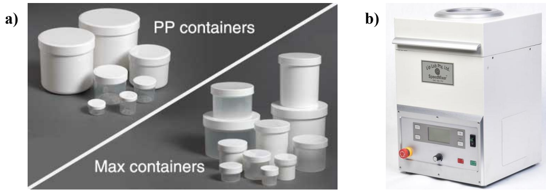
Figure 9.2 Mixing apparatus: Polypropylene containers (a), Hauschild Speedmixer DAC-150 (b)
