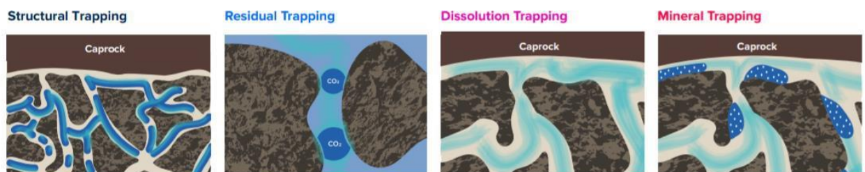
Figure 10 Trapping mechanisms during injection and storage of CO 2 . Source: IPCC 2005
