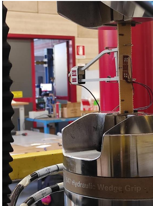
Figure 3-9: picture of a specimen tested with both strain gage (front) and extensometer (back)
