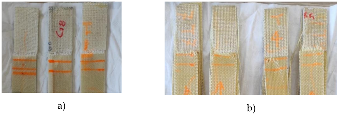
Figure 3-18: failure location of (a) glass and (b) Kevlar samples at clamping cite.
