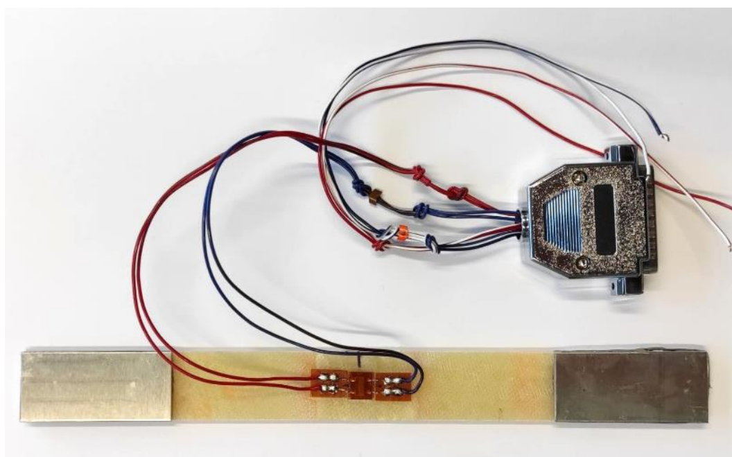
Figure 3-22: G8(L) tensile specimen with applied strain gages.
