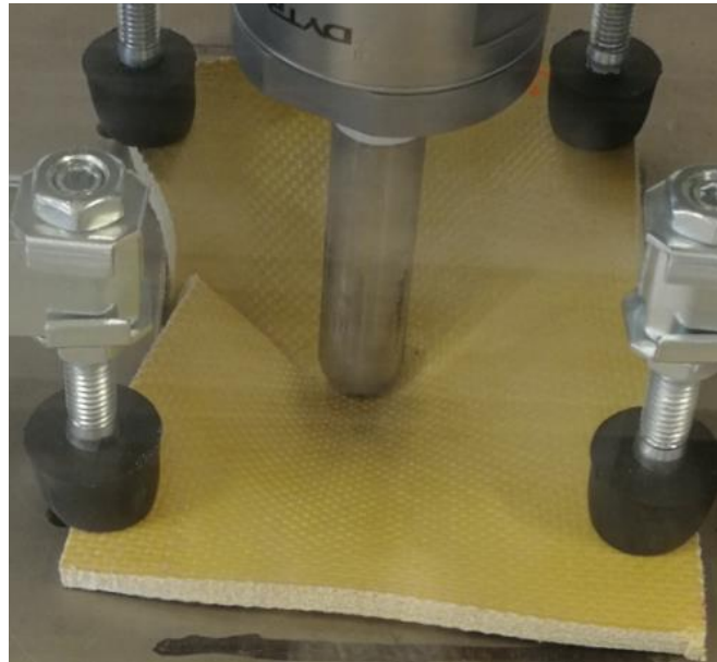
Figure 3-47: impacted panel after the test.
