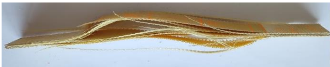
Figure 3-29: side picture of a failed specimen showing delamination.
