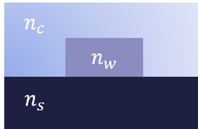
Figure 19: scheme of the cross section of strip WG (translationally invariant on the not shown direction). The refractive index of the WG made by a-SiN is n_w = 1.852 , then we distinguish two region s: the cladding ( n_c : H 2 O = 1.3296 PMMA = 1.4850281701926) and the substrate (if SiO 2 n_s = 1.454 ).
