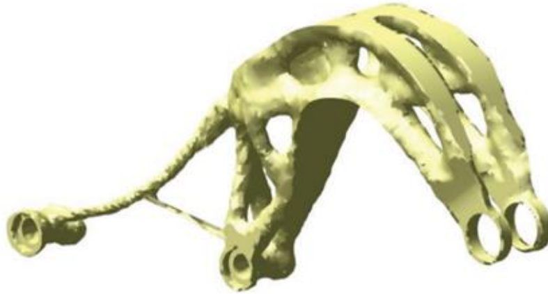
Figure 17. Raw results from the topology optimization. Needs post-processing.
