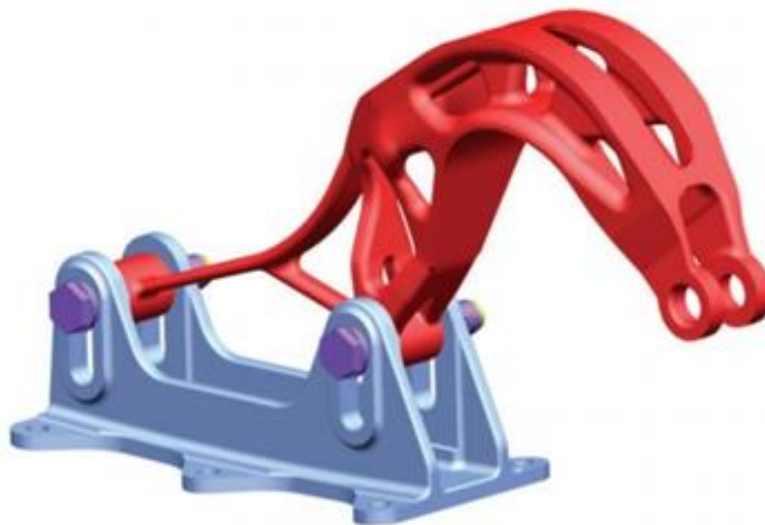
Figure 18. Final results of the topology optimization, after the post-processing is finished.
