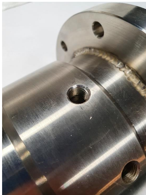
Figure 3.42: Detail of the two 1/8" NPT threaded holes in the Post-Chamber.
