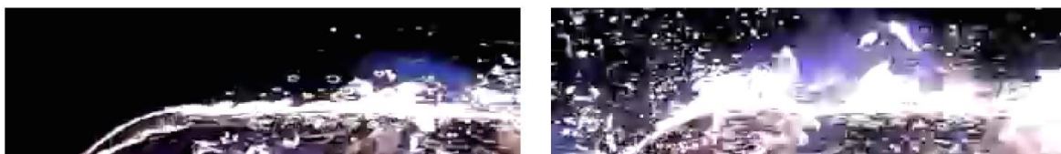
Figure 2.5: High-speed images of paraffin combustion at 4.9 bar. Nominal combustion (left) and blowing event (right) [20]. (Oxygen flows from left to right)
