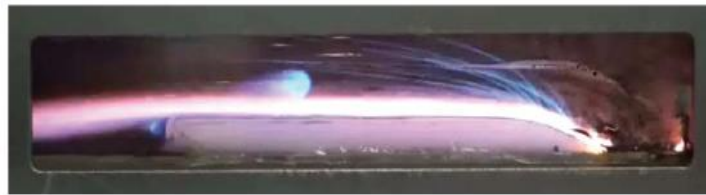
Figure 2.2: Combustion visualization of paraffin-wax FT-105 produced by Nippon Serio, having (on average) 51 carbon and 104 hydrogen atoms [24].
