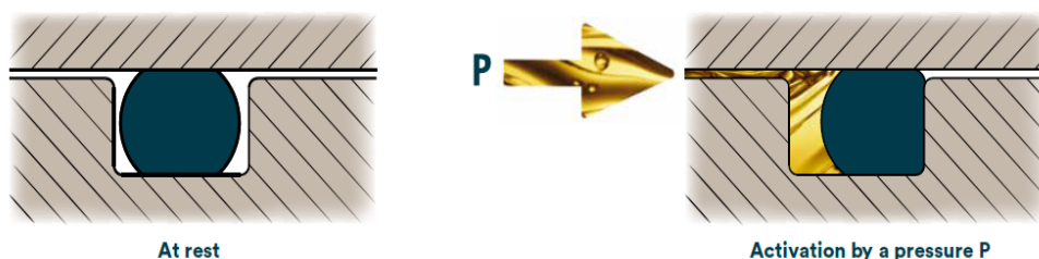
Figure 3.29: O-ring deformation caused by a pressurized fluid [39].
