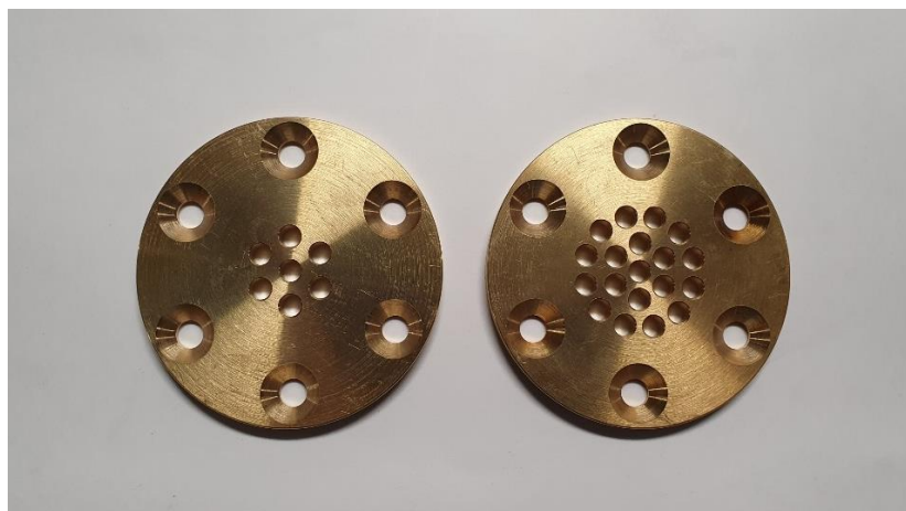
Figure 3.17: Picture of Injector Head A (left) and Injector Plate B (right).
