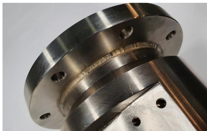
Figure 3.11: External welding, Main-Chamber.
