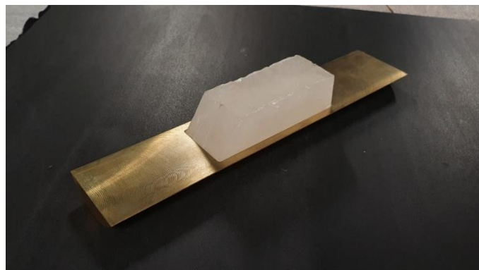
Figure 3.23: Picture of the paraffin grain positioned on the Grain Holder.
