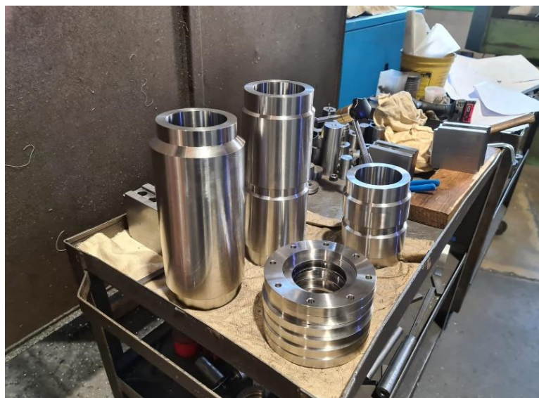
Figure 3.4: AISI 304L hollow bars during manufacturing.
