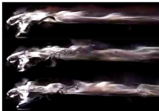
Figure 2.3: Progression of a roll wave in the liquid layer during an atmospheric pressure test [19]. (Oxygen flows from left to right)
