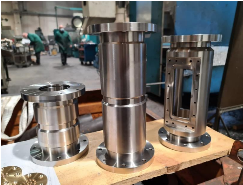
Figure 3.9: From left to right, picture of Post-Chamber, Pre-Chamber and Main-Chamber.
