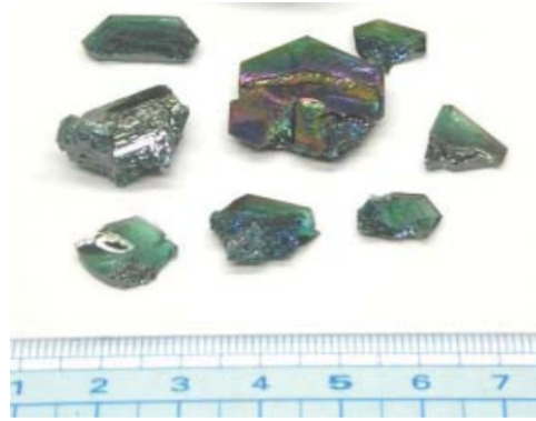
Figure 1.1: SiC fragments produced as secondary products during the Acheson process [39].
