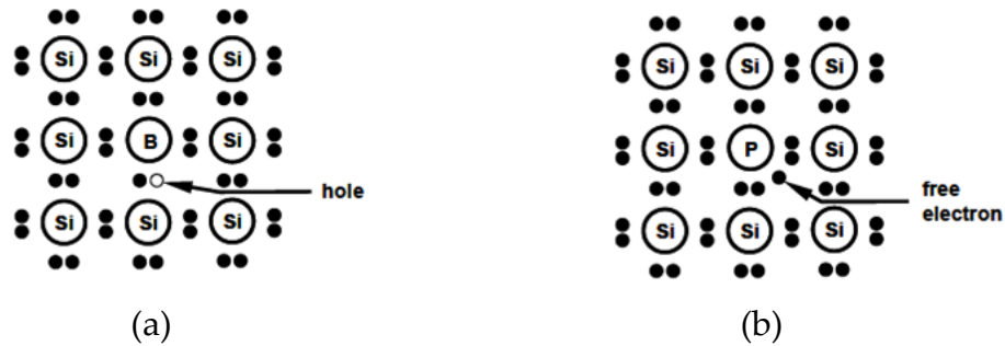
Figure 9: (a) P-type Material Example, (b) N-type Material Example
