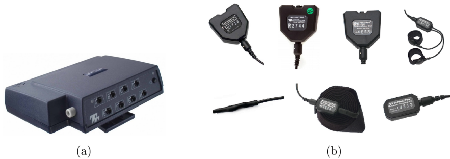
Figure 3.7: Procomp Infiniti (a) with a set of available sensors (b) top from left: EMG, ECG, EEG and SC. Bottom from left: body temperature, breathing and HBR
