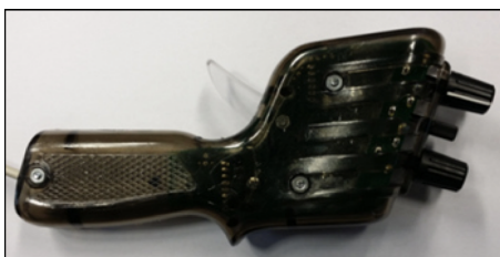
Figure 2.5: Lever used by passenger throughout autonomous drive to indicate the level of comfort in Scherer's study[39]
