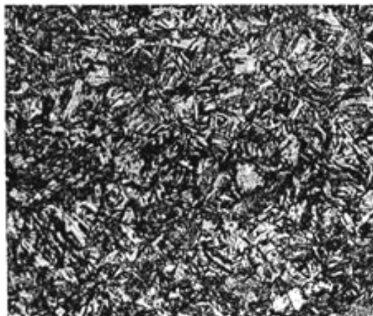
Figure 12. AISI 410 forging, hardened by holding 1h at 982°C and air quenched; finally tempered 2h at 566°C and air cooled. The resulting structure is tempered martensite and carbide; Vilella's reagent; 100X (20).
