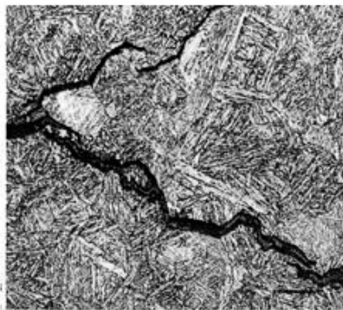
Figure 13. Martensitic stainless steel AISI 410 forged, hardened, tempered and finally etched in Vilella's reagent; 100X (20).
