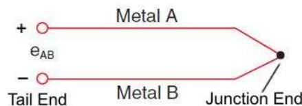
Figure 3.2.1.1. Sketch of a thermocouple.
