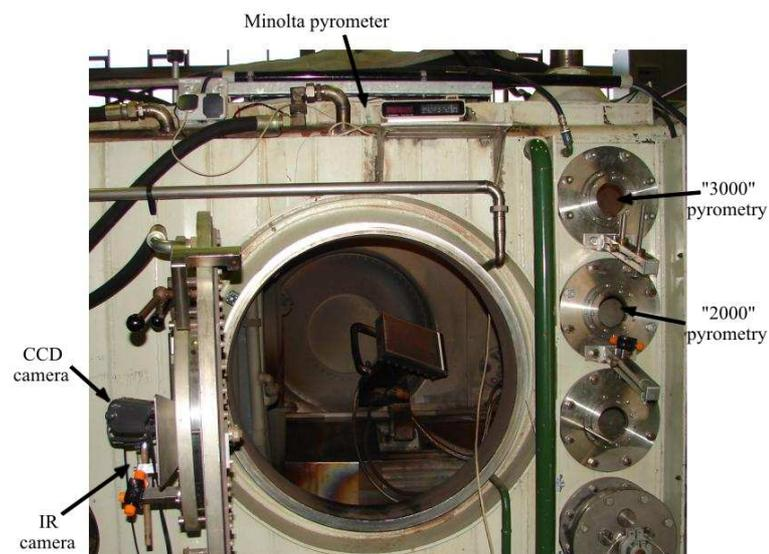
Figure 5.1.5. L3K test chamber. The small windows on the right provide the access to the pairs of pyrometers. The CCD-camera is visible at the access door.
