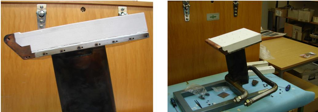
Figure 5.1.1. Investigated model (disassembled). Copper nose, steel support and KAPYROK are visible. Side view (left) and global view (right, also with cooling system pipes)
