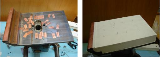
Figure 5.1.3. Positioning of the thermocouples. Installation on the base support (left) and positions after the integration of the KAPYROK (right).
